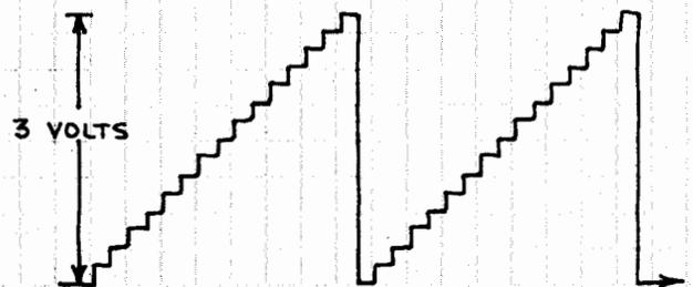
REMOVE C1 TO OBTAIN THIS STAIRCASE. FREQUENCY OF RAMP AND STAIRCASE IS 1/16 CLOCK FREQUENCY.
