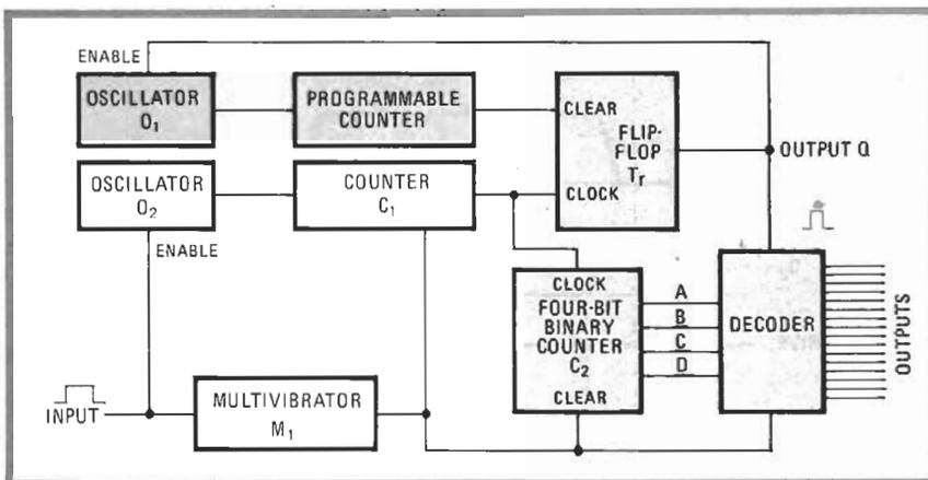
**1. Interval matching.** Simplified block diagram of the perpetual pulse-width counter (1a), which generates an output pulse only if the output pulses of M<sub>1</sub> and M<sub>2</sub> coincide in the AND gate G. The pulse chart (1b) shows the case when the duration of the input signal is equal to the developed interval.
