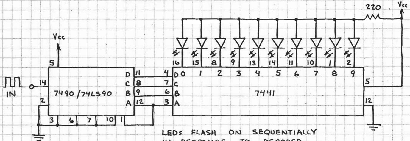
LEDS FLASH ON SEQUENTIALLY IN RESPONSE TO DECODED COUNT. ONLY ONE LED SERIES RESISTOR IS REQUIRED.
