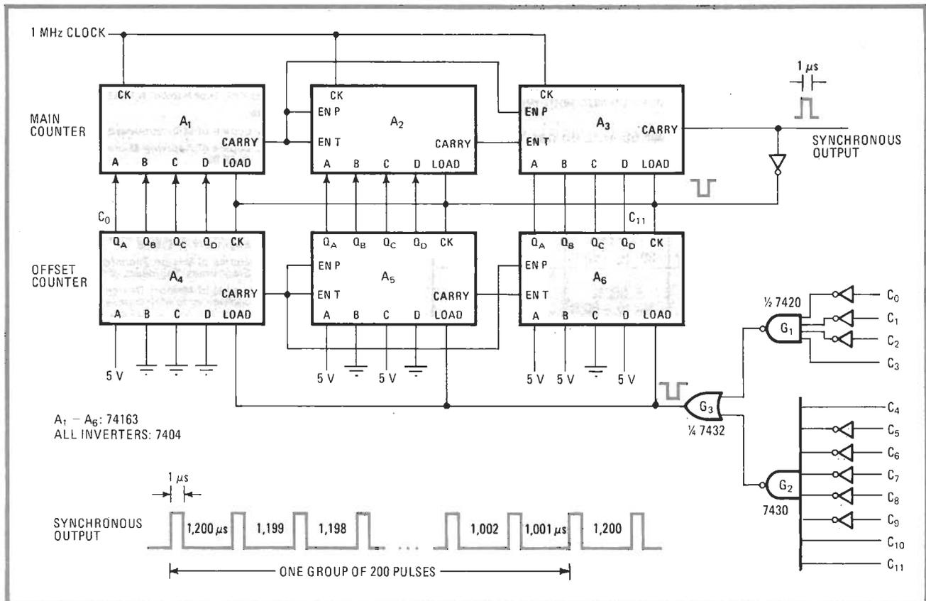
**Smooth staggering.** Two 12-bit counter chains generate a group of repeating  $N$  pulses spaced at  $(1,201 - M) \mu s$ , where  $M$  denotes the  $M$ th pulse of  $N$ , for incremental staggering of the radar-pulse rate. Master clock sets absolute value of maximum pulse-repetition frequency.
